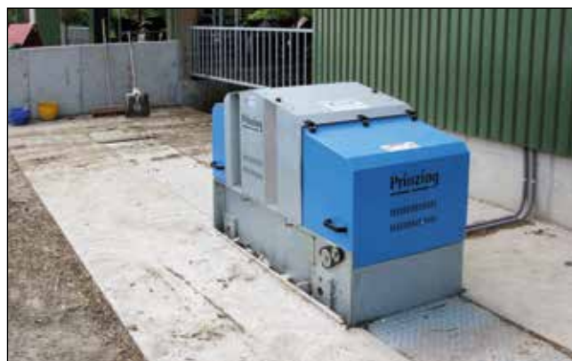
▲ Double drive winch DW7 with rope guidance system.
