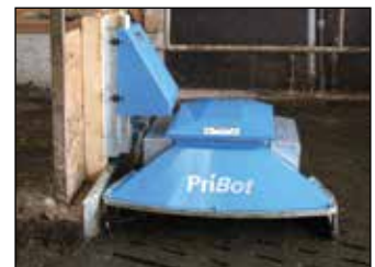
Automotive dunging robot PRIBOT
