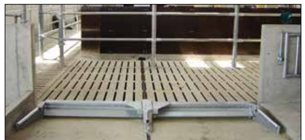
▲ PKSF for clearing on partial areas with slatted floor
