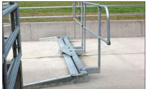
▲ Flap scraper PKSf with driving gate
