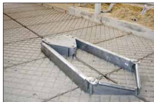
▲ Multi folding scraper in reverse motion
