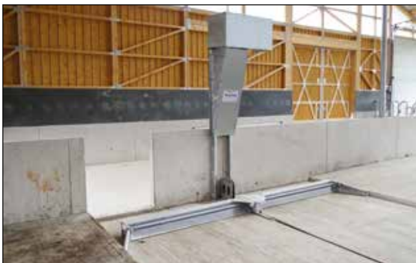
▲ Mounting the EW4 drive winch with wall bracket
